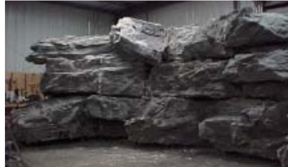
URESTONE panels produced by spraying a structural polyurethane / polyurea system into a real rock mold are attached to a modular support frame system.
