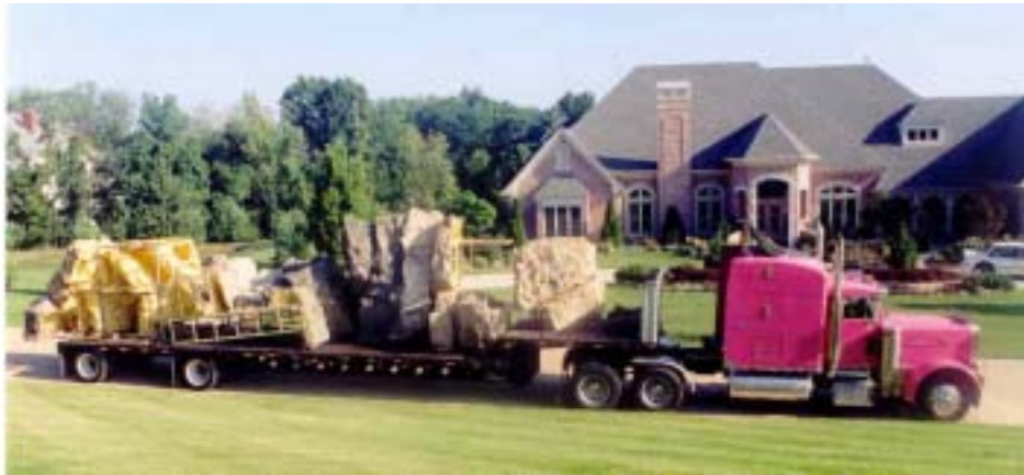
The rock feature is cut into modular sections and shipped on a flat bed truck. A key advantage of this system is that it is the lightest weight rock system available which makes shipping and handling relatively easy.
